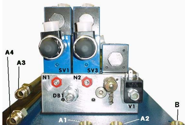
pic.3: hydraulic bloc
