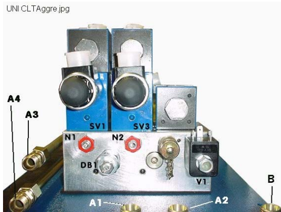
pic. 5: SV1 & SV2 position of the double seat valves
