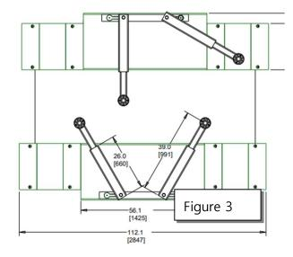
and complete contact with the ground. If there are gaps between the frame and the floor, those areas in which the load of the lift is passed to the base frame must be filled with high strength grout.
